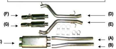
Note: anti-seize should be applied to all fastener threads, pipe slip joints and mating surfaces of ball /socket connections.
